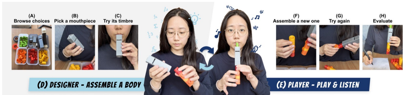
Figure 1: FlueBricks and the designer–player loop. FlueBricks is a construction kit of 3D-printed building blocks for building and customizing flute-like instruments. This figure illustrates the designer–player loop : users iteratively switch between designing instruments and playing them to form, test, and refine acoustic behaviors. (A–C) Users browse tangible building blocks that embody aeroacoustic properties, select a mouthpiece, and breathe into it to hear the sound it generates. (D) As designers, they connect modules to assemble a resonator body. (E) As players, they immediately test the sound by playing. (F–H) Based on what they hear, users reconfigure tangible modules to test new hypotheses (F&G) and play again to evaluate the sound effect (H). Through these iterations—hypothesizing, configuring, playing, and refining—users engage in acoustic reasoning .
